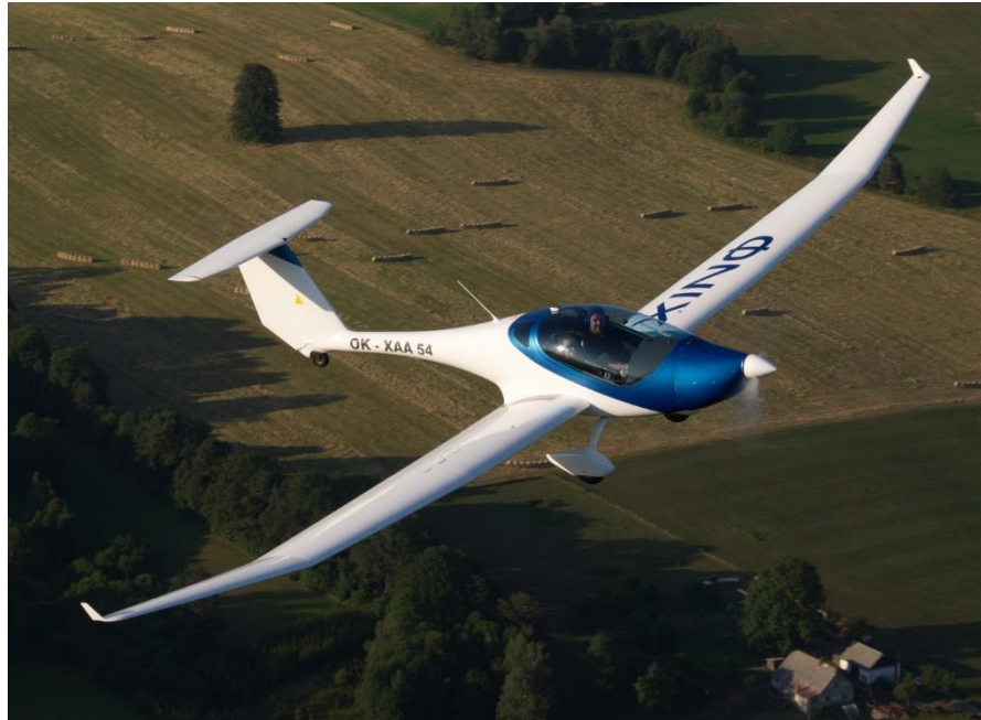
ΦNIX - Electro powered airplane with range extender
